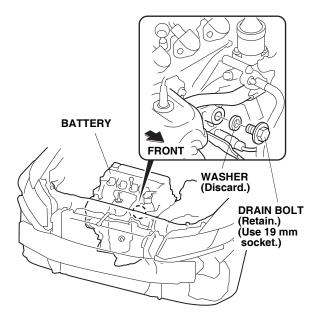
Install the engine block heater with aluminum washer into the bolt hole using a 24 mm socket and a torque wrench. Torque the engine block heater to 60 N·m (44 lbf·ft).
